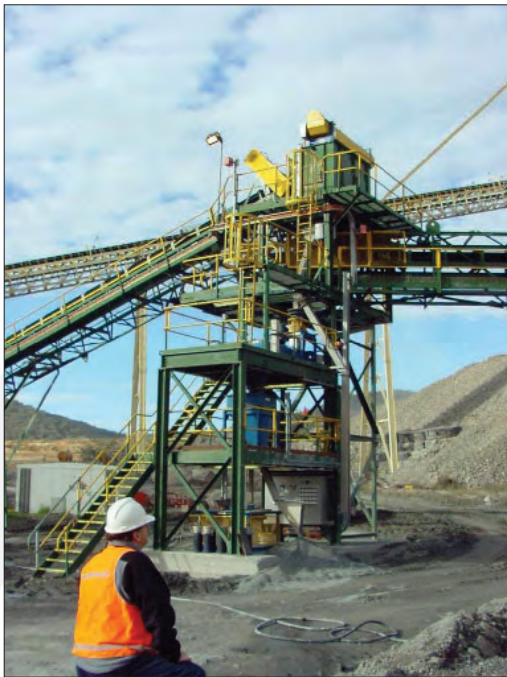
Knowing the delivered head grade is not straightforward – this is a sampling tower at a copper-gold mine
